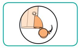
9. Lock all the wheels by pressing down the brake lever on each wheel.
