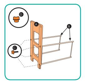
1. Attach an end panel (A) to the two side frames (B) using bolts (C) and then tighten using tool (D).
