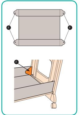
5. Place the base shelf across the side frame's lowermost tubing. Wrap flaps (F) around the upright tubing of the two side frames and secure using press studs.
