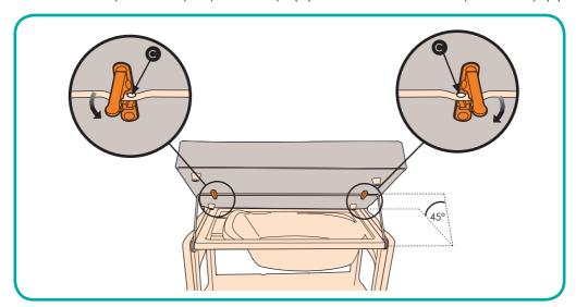
8. Standing at the back of the changing unit, angle the hinged wire frame up to  $45^{\circ}$  and clip the padded top on ensuring the two metal pips (C) are positioned on the inside of the clips. Fasten the clips and lower the padded top.
