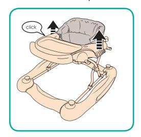
2. **To close:** Hold the front of the walker and at the same time, turn and pull the locking mechanism forward and lower the upper part of the walker all the way down.
