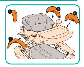
2. Match the number on the underside of the mudguard with the number on the walker body.
