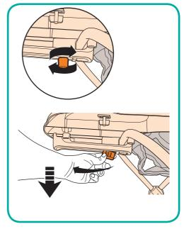
3. **To adjust the height:** The simplest method to adjust the height is to lower the upper part of the walker all the way down (as above, in step 2) then pull the upper part of the walker back up so that it clicks into one of the three height positions.
