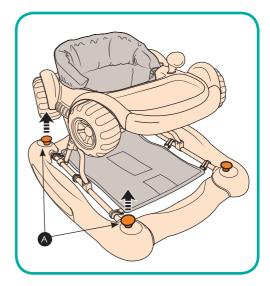
2. Whilst pulling up on both locking knobs, turn the base 90 degrees upwards into the rocker mode. Repeat on the opposite side and check that both sides of the base are locked in position.
