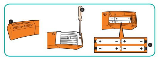
2. **Battery operation:** The battery compartment is located on the underside of the base and can found by the diagram (i) printed at the end of the right-hand base arm.
