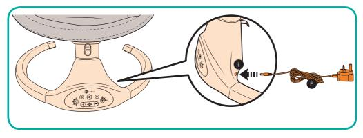
1. **Mains operation:** Insert the round-pin end of the power adaptor (F) into the round socket at the rear of the rocker base (i).
