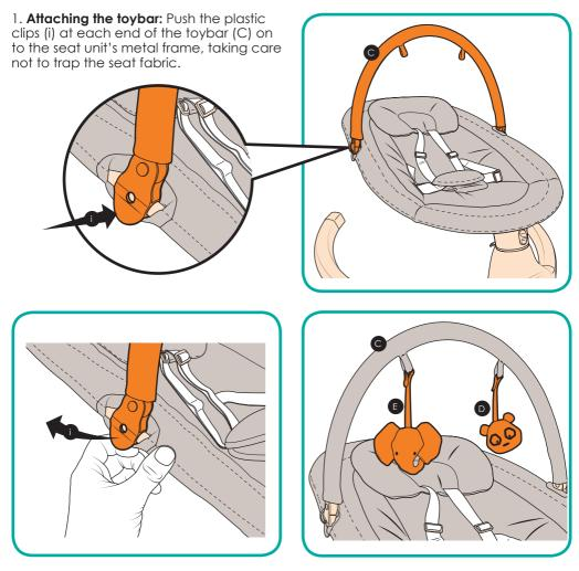
2. To remove the toybar: using your thumb and forefinger prise the plastic clips (i) outwards off from the seat unit frame.
