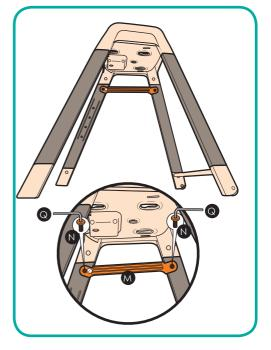
6. Attach leg side-brace (M) using two Allen bolts (N). Tighten the bolts using Allen key (Q). Attach the remaining second leg side-brace in the same way.
