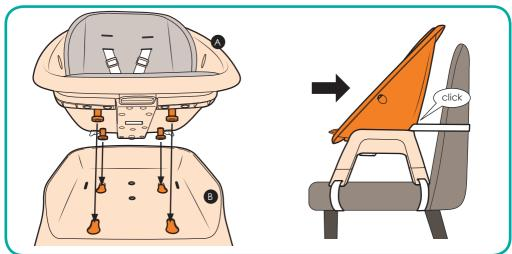
5. Insert the four pins on the underside of the seat shell (A) into the four keyhole slots on the upper surface of the seat base (B) and push the seat shell back into the seat base to lock the four pins in place.
