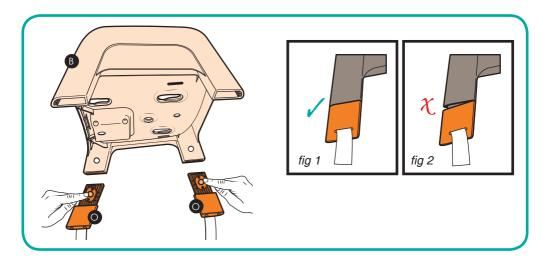
1. Press in button (i) and slide the booster-seat feet (O) into the sockets on the seat base (B), ensuring each foot 'clicks' into place. Attach all four feet and check that they are all properly connected.
