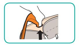
14. Whilst pulling the lever on the frontunderside of the seat, push the armrest down so that it locks into the seat.
