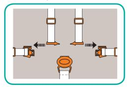
1. Place the crotch strap between your child's legs and slide the shoulder strap clips onto the waist strap clips.
