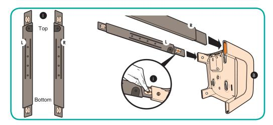
1. Attach the two front legs (I) (legs with long slots) to the stool top (B) as shown. The left leg (L) goes in the front left socket and the right leg (R) in the front right socket. Press in button (i) at the top of each leg and slide the legs into their sockets on the stool top, ensuring the legs 'click' into position.
