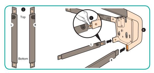
2. Attach the two rear legs (J) (legs with NO slots) to the stool top (B) as shown. The left leg (L) goes in the rear left socket and the right leg (R) in the rear right socket. Press in button (A) at the top of each leg and slide the legs into their sockets on the stool top, ensuring the legs 'click' into position.
