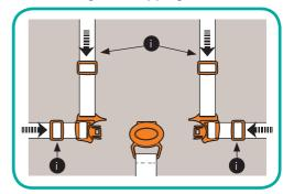
2. Insert the harness clips into the buckle, making certain your child's fingers are clear. Adjust the sliders (i) on the waist and shoulder straps so that the harness fits snugly.
