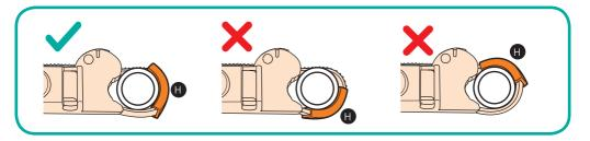
3. Ensure the gripper pad (H) is positioned correctly to provide the best grip and protection regardless of tube diameter.
