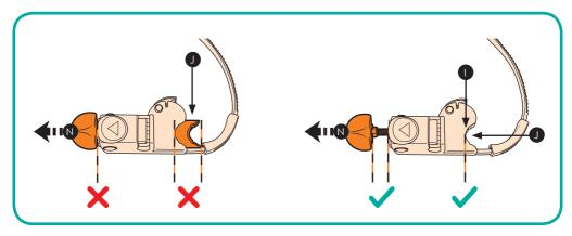
2. Unscrew block screw (N) until the block (J) is fully retracted as in Fig2. Block (J) should be flush with the connector body (I), if it is sticking out then push it in.
