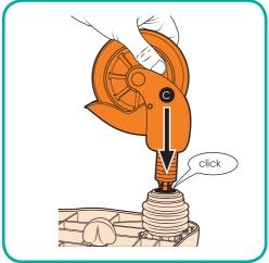
2. Align the wheels (C) to the wheel housing and push the wheels firmly into the housing unit until you hear a "click".
