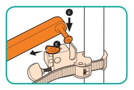
1. Slide out the quick release buttons (K) and insert the arm pins (ii) into the connectors.
