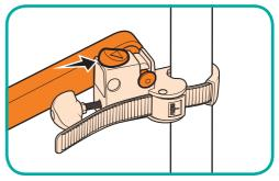
2. Slide back the quick release buttons to lock the arm pins in place.
