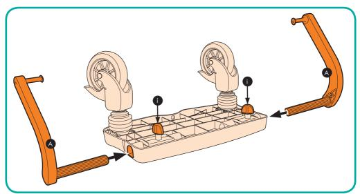
3. Loosen screws (i) enough until you can easily insert and rotate support arms (A).
