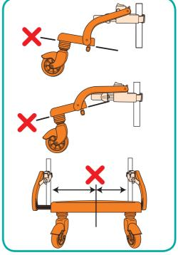
**IMPORTANT:** If the board is not central or not level then adjust the board and arms or reposotion the connectors until everything is correct.
