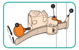
2. Ensuring both connectors are at the same height and gripper pad (H) is positioned correctly (see step 3 below for details), tighten block screw (N) as far as possible until block (J) is tightened fully against the leg tubing.
