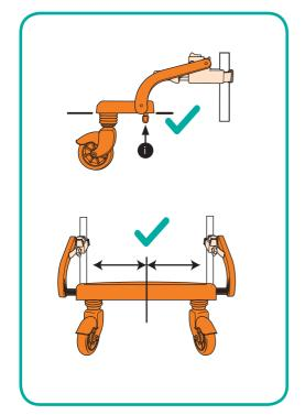
3. Adjust the board so it is both central between the two arms and level. Tighten the screws (i) underneath the board to lock the board into position.
