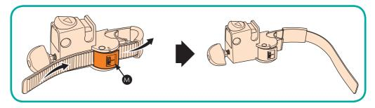
1. To get the connectors ready for fitting on the pushchair, press the strap lock (M) and release the strap (L).
