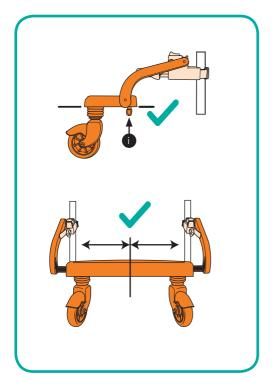
3. Adjust the board so it is both central between the two arms and level. Tighten the screws (i) underneath the board to lock the board into position.
