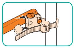
2. Slide back the quick release buttons to lock the arm pins in place.
