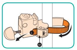
1. Pass strap (L) around the chassis tubing and through strap lock (M). Pull Strap (L) as tightly as possible through
