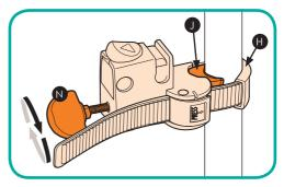
2. Ensuring both connectors are at the same height and gripper pad (H) is positioned correctly (see step 3 below for details), tighten block screw (N) as far as possible until block (J) is tightened fully against the leg tubing.
