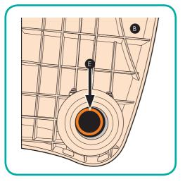
1. Place the buggy board platform (B) upside down on a sturdy surface. **IMPORTANT:** If the washers (E) are loose in the box, or in the bag with the storage strap, place them into the wheel housing as shown in the picture.
