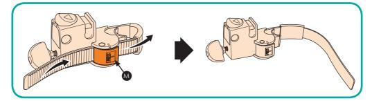
1. To get the connectors ready for fitting on the pushchair, press the strap lock (M) and release the strap (L).
