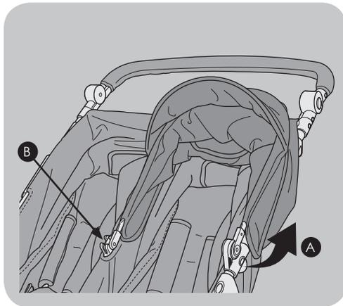
2. **Remove the hood:** Unfasten the press studs on the back of the right-hand hood. Unclip the hood-clip (A) and pull the round connector from the mounting point (B).
