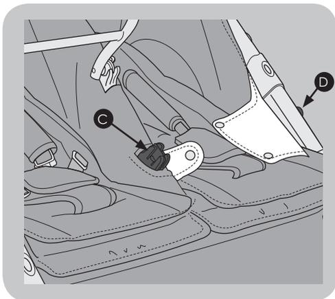
3. **Expose the two lower mounting points:** Unfasten the press stud on the fabric covering the lower-centre mounting point (C). Unfasten the two press studs on the fabric covering the lower-right stud (D).
