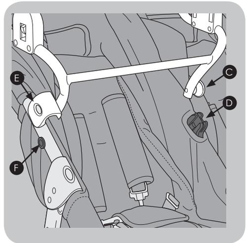
4. Push the round connector (C) on the car seat adaptor into the mounting point (D). Connect the clip (E) over the stud at point (F).
