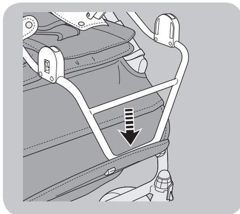
4. Place the bottom bar of the car seat adaptor onto the footrest of the stroller.
