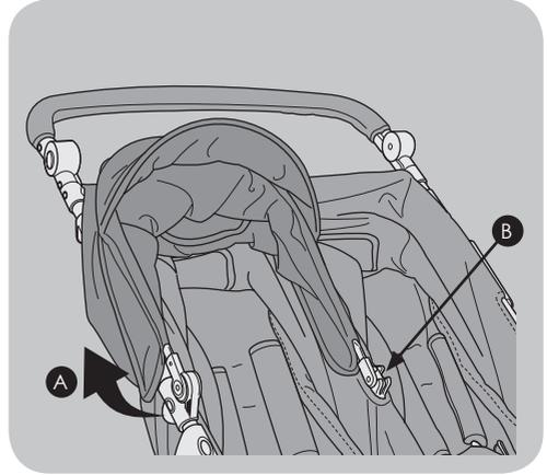
2. **Remove the hood:** Unfasten the press studs on the back of the left-hand hood. Unclip the hood-clip (A) and pull the round connector from the mounting point (B).
