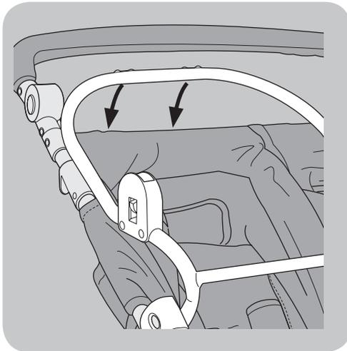
3. Place the two hooks on the car seat adaptor over the top of the stroller chassis.
