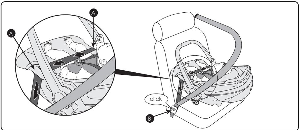
Place the vehicle lap belt across the child car seat and slide the lap belt into the slots (A) on both sides of the child car seat. Buckle up the vehicle seat belt (B).
