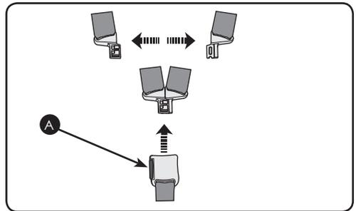
Feed the straps through from the front of the seat out to the back.
