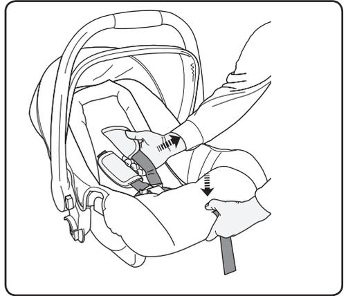
Press the red release button (A), unbuckle the harness, move the shoulder straps apart and remove the shoulder pads.
