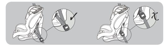
With your child car seat now buckled in, check it is secure by pulling forward from both harness straps, there should be little or no movement. Next check that the vehicle's seatbelt buckle is **NOT** resting against the child car seat shell. This is called 'buckle crunch' and could cause the child car seat to work loose or the seatbelt to come undone in an accident. If you find you are experiencing 'buckle crunch' then this child car seat is not suitable for your vehicle.
