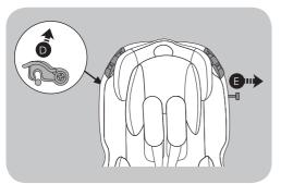
Release catch (D) on the top left hand side of the shell and remove the installation bar (E).
