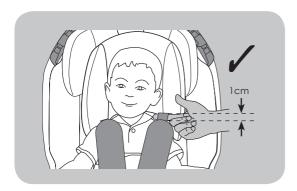
The harness should allow 1 fingerwidth (1cm) of space at the top of the shoulders. This is the ideal tightness.
