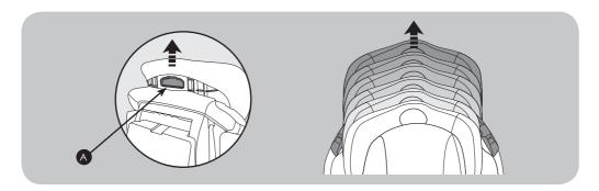
Adjust the headrest by pulling the adjuster handle (A) on the back of the headrest and raising or lowering according to your child's height.
