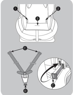
Insert waist strap retainer buckles (C) through the two slots (1) and (2) on the cover and out through the outer slots on the back of the shell then back through the inner slots.
