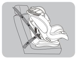
Feed the seatbelt between the shell and the base and ensure the seatbelt is not twisted.
