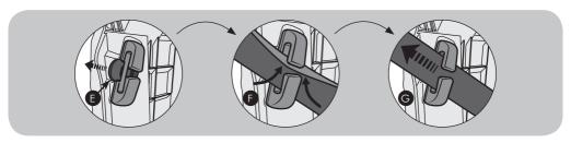
To operate the lock-off device: Pull down on tab (E) to open the locking device. Feed the seatbelt into the gap between the tab and the locking device (F). Pull the diagonal section of seatbelt tight (G).
