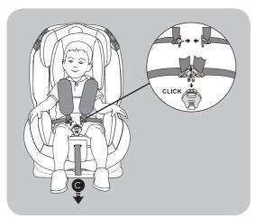
After placing your child in the child car seat, match the two halves of the harness buckles together and insert them into the crotch buckle. Make sure the shoulder straps fit your child snugly by pulling the adjuster belt (C).
