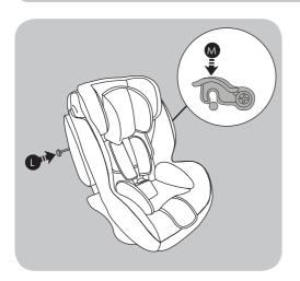
Return the shell to its original position and re-insert the installation bar (L) and secure lock (M).
