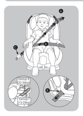
Place the seatbelt shoulder strap through the most suitable belt guide slot (A): Use the lower strap hook for children in group I [15 - 25kg].
