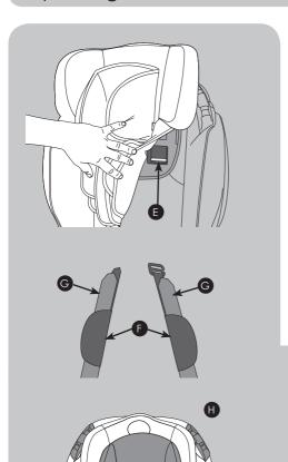
Adjust the headrest so that when you lift up the headrest fabric you are able see the metal bar (E) through the backrest. Slide the shoulder pads (F) over the shoulder harness straps (G), ensuring the seams of the shoulder pads are facing outwards.
