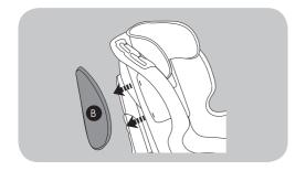
Pull the two (SAP) Side Armour Protection systems (B) in the direction of the arrows to unclip them from the shell and remove their covers.
