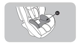
Remove the booster cushion insert (M) from the crotch strap.
