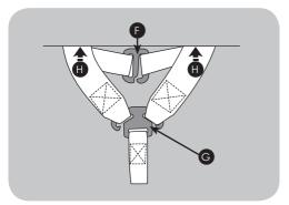
Unhook the shoulder pad straps from shoulder pad connector (F). Unhook the shoulder harness straps from yoke (G).
