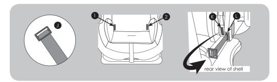
Locate the two metal retainer buckles (J) under the seat cover at points (1) and (2). Pass the metal buckles on the waist harness from the front of the shell, through the inner slots (K) on the back of the shell and back out the outer slots (L), to the front to remove the harness.
