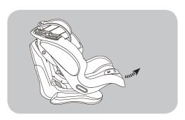
Pull the recline adjuster handle under the front of the shell and whilst holding it, pull the shell forwards to its most reclined position.
