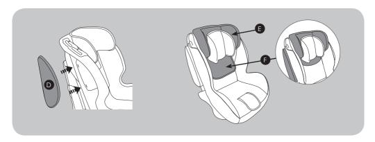
Stretch the side covers over the two (SAP) Side Armour Protection systems (D) and clip them back on to the shell. Once clipped on jiggle them to ensure the are firmly clipped on.
