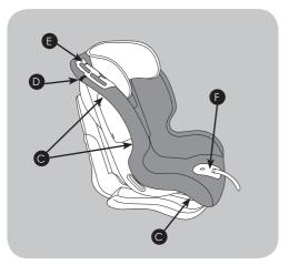
The main cover is held in place by a series of hooks (C) located on the back and underside of the shell. Unhook the cover's elastic from the hooks. Undo the Velcro® tabs (D) on the shoulders of the shell, work the cover from under the strap hooks (E) and from around the plastic adjuster panel (F) and remove the cover.
