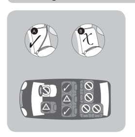
The child car seat can only be used with an automatic 3-point safety belt (A) and **NOT** with a 2-point lap belt (B).
