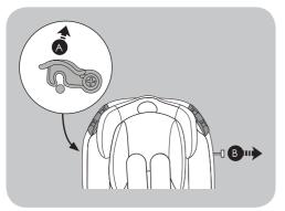
Release catch (A) on the top left hand side of the shell and remove the installation bar (B).
