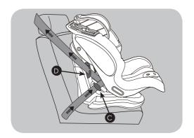
Thread the horizontal lap belt section under both hooks (C) and remove all the slack by pulling up on the diagonal section of seatbelt. Thread the diagonal section through the lock off device (D).
