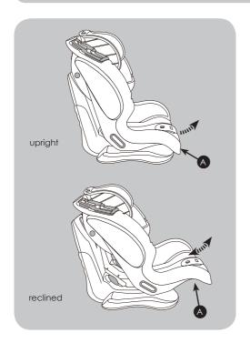
The child car seat can be used in four different seat positions, from seated to a reclined sleeping position. Pull the recline adjuster handle (A) under the front of the shell and pull the shell forwards or backwards, release the handle on your required position when hearing a distinct click.
