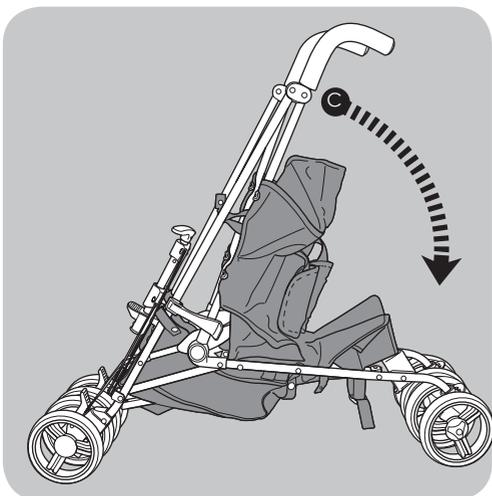
3. Hold both the handles and gently fold the stroller forwards (C) until it is fully folded. Do not force it down. If it does not go down then check for obstructions and repeat actions in steps 1 & 2 above.
