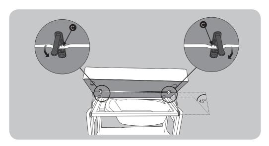
8. Standing at the back of the changing unit, angle the hinged wire frame up to 45° and clip the padded top on ensuring the two metal pips (C) are positioned on the inside of the clips. Fasten the clips and lower the padded top.
