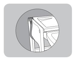
14. The drainage hose can be left attached to the outlet on the underside of the bath tub. The free end of the hose can be hooked onto the side panel.
