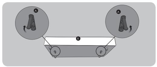
7. To attach the padded top: Open the clips (A) on the underside of the padded top (B).
