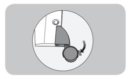
9. Lock all the wheels by pressing down the brake lever on each wheel.
