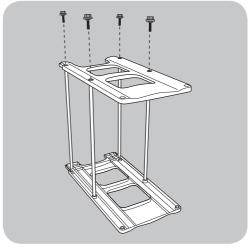
2. Place the changing unit on its end and loosely attach the other end panel using four bolts.
