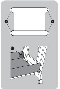
5. Place the base shelf across the side frame's lowermost tubing. Wrap flaps (F) around the upright tubing of the two side frames and secure using press studs.
