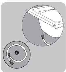
13. To empty the bath, connect the drainage hose (B) to the outlet on the underside of the bath tub and drain the water into a bucket.
