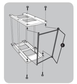
3. With the changing unit on its end, place the ends of the top frame (E) into the sockets on the inside of each end panel. Secure with two bolts, then carefully turn the changing unit over and secure with two more bolts.
