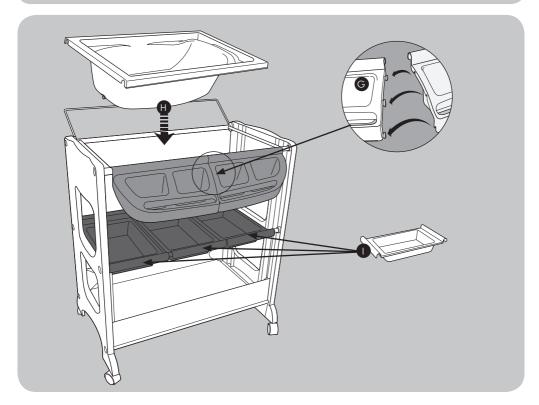
6. Clip the two side trays (G) together and then hook over the front of the top frame. Place bath tub (H) into the top frame, hooking it over the top frame and the side trays(G).
