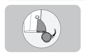
11. Lock all the wheels by pressing down the brake lever on each wheel.
