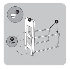
1. Attach an end panel (A) to the two side frames (B) using bolts (C) and then tighten using tool (D).
