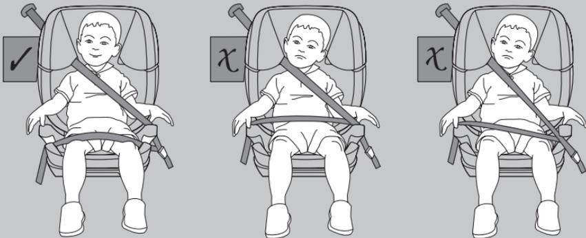
Make sure the lap belt passes under the armrests through the lap belt guides and that the shoulder belt passes diagonally through the shoulder belt guide and over the armrest nearest to the seat belt buckle.
