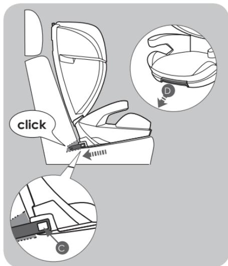
Position the child car seat on the selected passenger seat and slide the child car seat back till the connectors lock onto the ISOFIX points in your vehicle.
