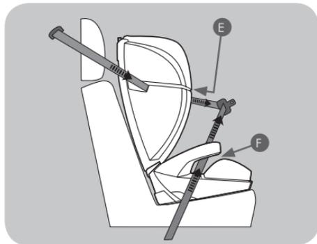
Slot the vehicle seat belt's shoulder strap through the shoulder guide (E) and the waist strap under the armrest (F).
