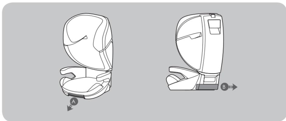
Pull the release handle (A) and at the same time pull out the recline block (B).
