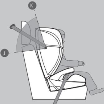
Ensure the vehicle seat belt is positioned in the arc between (J) and (K), failure to do so may result in the seat belt laying incorrectly across your child and reducing the safety of the seat.
