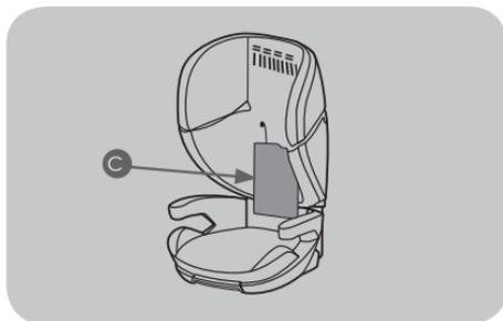
Remove the small seat back cover by unhooking the elastic loops, starting at the top.
