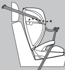
Remove the vehicle seat belt from the belt guides.
