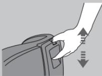
Adjust the child car seat to the correct height by pushing the backrest adjusting button and moving the backrest up or down to the desired height.
