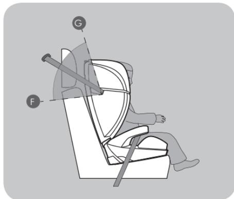
Ensure the vehicle seat belt is positioned in the arc between (F) and (G), failure to do so may result in the seat belt laying incorrectly across your child and reducing the safety of the seat.
