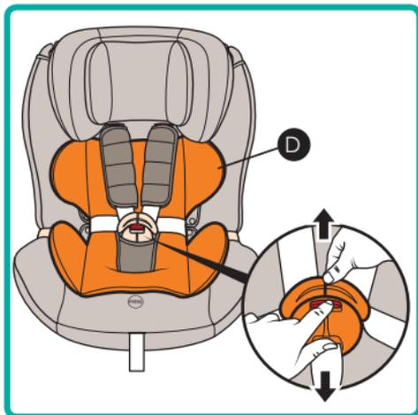
7. Release the 5-point harness buckle (See "Using the 5-point harness" on pages 10-11 for details) and remove the insert cushion (D).
