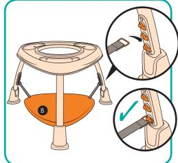
1. Remove the 3 straps (A) from their storage positions (i) on the underside of the footpad/table top (B)
