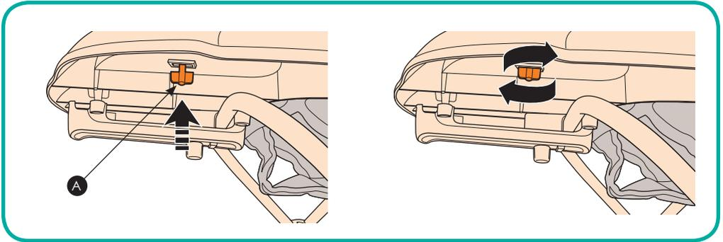
3. Secure the toy tray to the walker body by pushing the tabs (A) on the underside of the walker body, into the corresponding holes in the toy tray and then turning the tabs to fix the tray in position.
